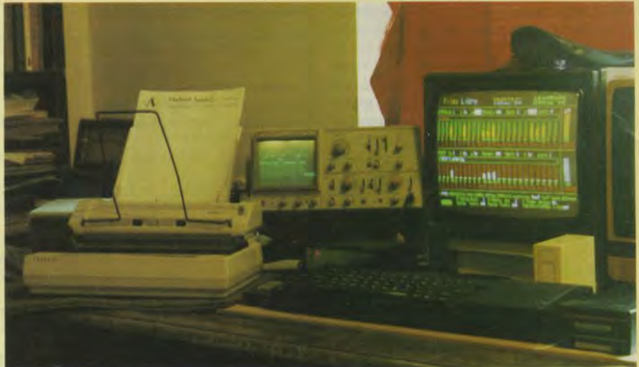
My system: the oscilloscope is displaying output for the lighting dimmer racks, the small box behind and to the left of the QL is the dimmer-board interface, the fireman's cap is used to protect against morning sun through the windows!
